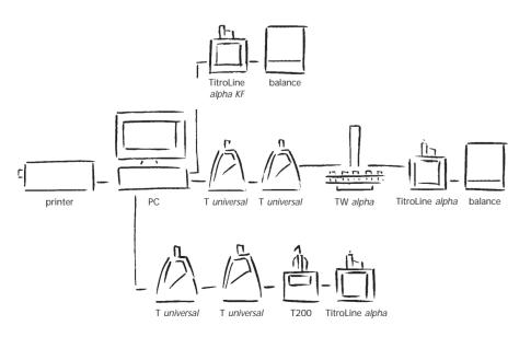
sample changer TW alpha, for example, is controlled by the software. For more complex titration tasks including sample preparation, the connected burettes take over the required dosing tasks first and then the titration is carried out with the TitroLine alpha. It is, of course, also possible to use the software exclusively for dosing operations The following diagram shows you examples of possible equipment combinations
