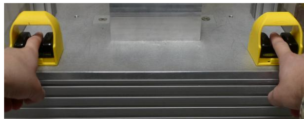
Figure 1 – To operate the test bridge, ensure test chamber is safe to close and all extremities clear of the test chamber. Once the test bridge is confirmed safe to operate, place both fingers into the finger-operating switches simultaneously to initiate the test bridge. Fingers must remain within the finger-operating switches for the test to initiate. Removing fingers will cause test chamber to return to the UP position.
